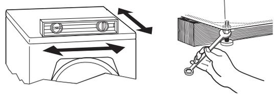
If the washer is against a wall, move the washer out slightly before tipping back. If the washer is not level, first prop the front with a wood block and adjust the feet as necessary; then prop the back and adjust feet as necessary. Repeat this step until washer is level.
